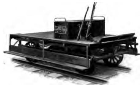
Buda No. 14-W. Bridge Gang Motor Car
